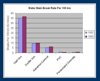
Final Water Mains Break Data on Different Pipe Materials for 1992 and 1993, NRC Canada
