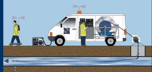
Tethered inline leak location – proven sensitivity
